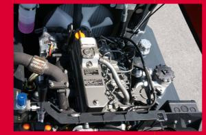
Smooth running Yanmar engins, accessible by 3 sides thanks to the operator's platform tiltable to the rear by 90°.
