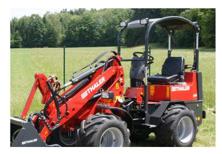
Hydraulically in height adjustable 4-post-**Rops-Fops protection** cage.
