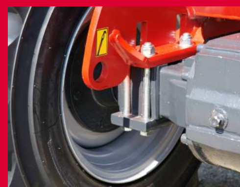
Full cast axle for ideal thrust capacities
